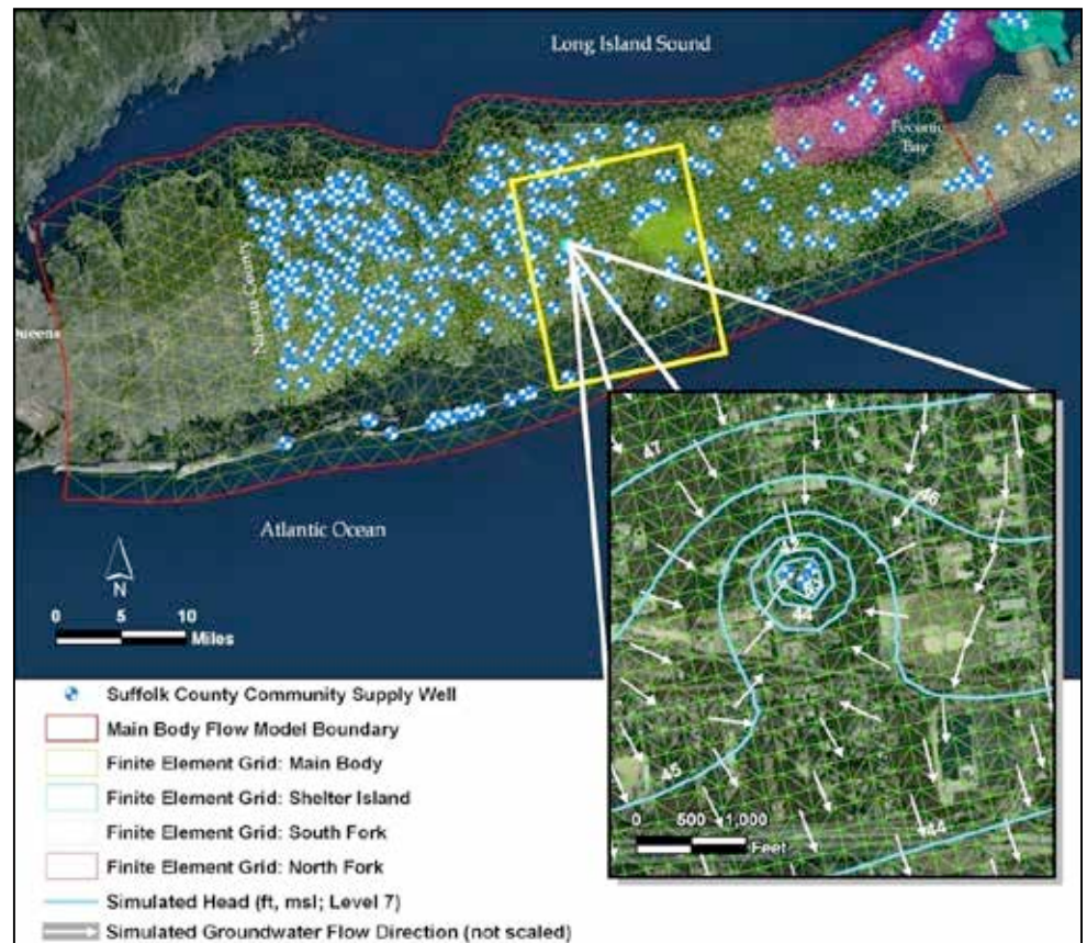
Figure ES-1 Calibrated three-dimensional groundwater and salt water intrusion models were used to develop source water assessments for each community supply well, to help to understand the relationships between land use and groundwater quality and groundwater and surface water resources.
